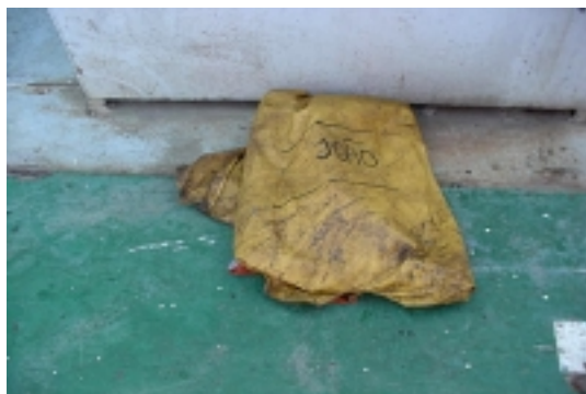
Photo 02 – Pig rib covered with sail cloth Kevlar® suit and yellow PVC cloth. We named the test speciman:John (João)
