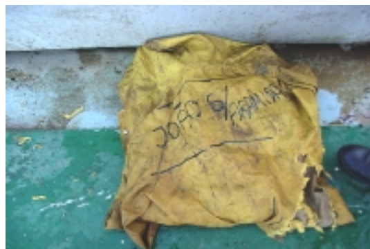
Photo 09 – John ( João ) is prepared for the UHP test using only PVC and sail cloth
